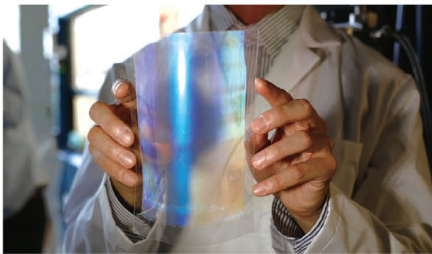
'Block copolymer,' produced by Hiroaki Sai and Ferdinand Kohle from the Wiesner Group, refracting various wavelengths of light dependent on the angle from which it is viewed.
